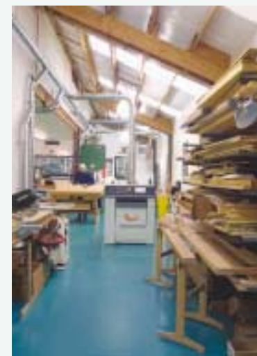
Efficient layout. Machines are arranged so that wood progresses in logical order from the lumber rack through all of the workstations.
